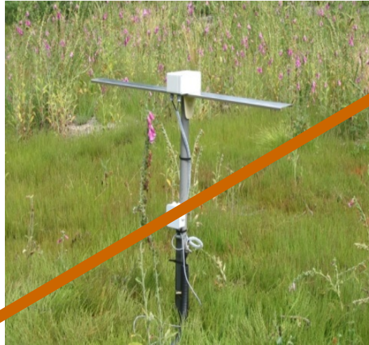
Active Short Fat Dipole (2006) length = 1.21m Height = 1m 50E/Antenna
