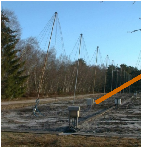
Log-Spiral Antenna (2005) Circular polarization Diameter = 5m Height = 6m
