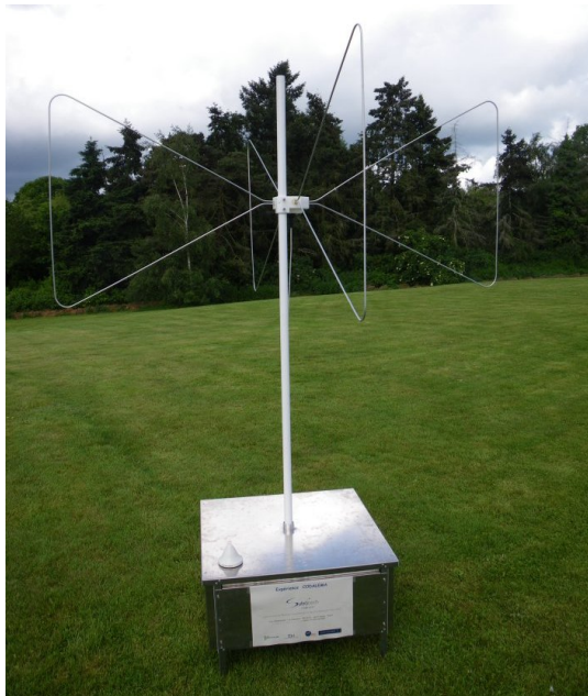
Figure 10: The new autonomous station. It features a dual polarization antennas hold by a container hosting the on board electronics.
