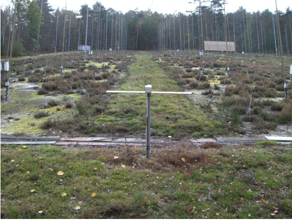
Figure 2: One of the short dipole antenna in front of the logarithmic antennas of the DAM. The shelter housing the detector power supplies and the DAQ system appears at the back left of the picture.
