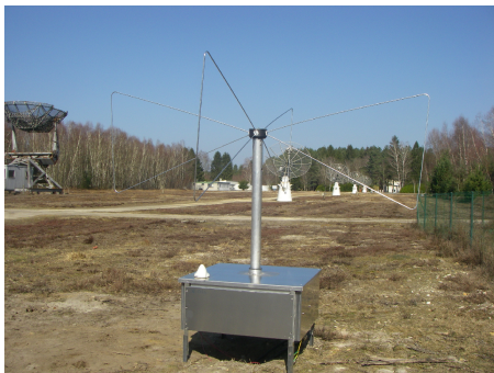
Figure 1. A butterfly antenna on the field at the Nançay Observatory.
