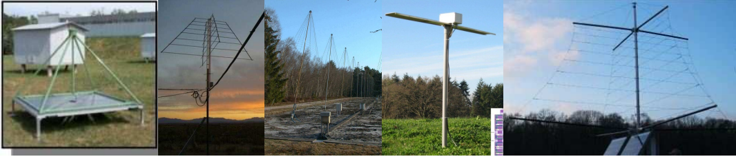
Figure 1: Some of the various antennas used on the current cosmic ray air shower radio detection experiments. From left to right: antenna from LOPES, Log Periodic Dipole Antenna (LPDA) used on LOPES STAR , Nançay Decametre Array (DAM), CODALEMA active dipole and a LPDA used at Auger.
