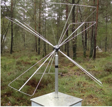
Figure 3. The tri-pole antenna.
