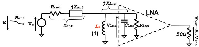
Shunt input inductance Ls parallel to the LNA input impedance
