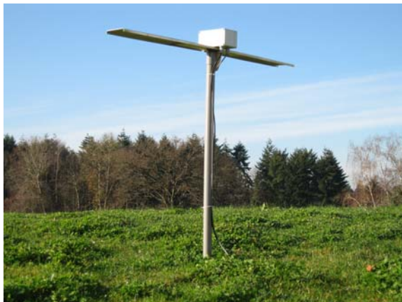
Fig. 2: View of the new broadband antenna with its front-end amplifier box used since 2006.
