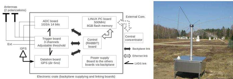
**Fig. 1. Left:** Schematic description of the station elements. **Right:** A butterfly antenna on the field at the Nançay Observatory.
