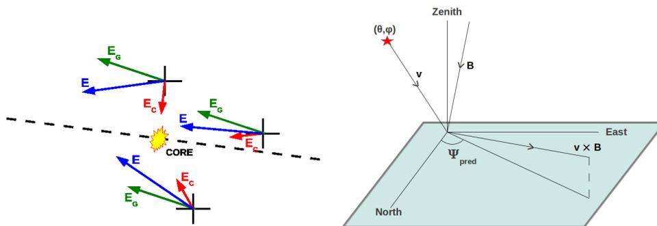
**Fig. 3. Left:** Illustration of the dependance on the relative position of the antenna with respect to the shower axis (dashed line) of the total intensity of the electric field (blue) due to the charge excess (red) and the geomagnetic (green) contributions. **Right:** Definition of the predicted polarization angle.
