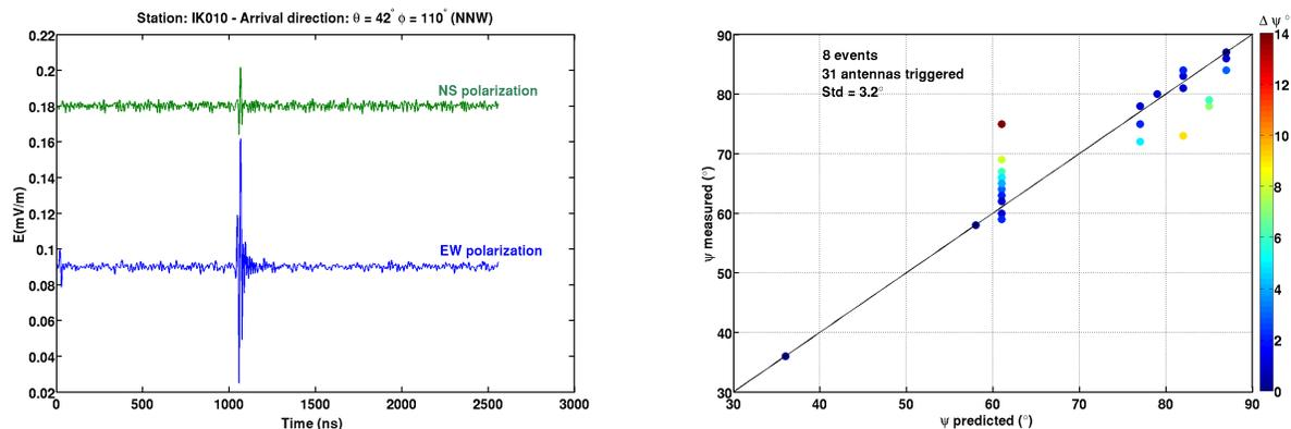
**Fig. 4. Left:** Wave shape for both East-West and North-South horizontal polarizations of the electric field filtered in the 30-80MHz band. **Right:** Polarization angle  $\psi_{pred}$  calculated according to  $\vec{v} \times \vec{B}$  as function of  $\psi_{meas}$  deduced from the antenna signals. The angular difference  $\psi_{meas} - \psi_{pred}$  are represented by colors.
