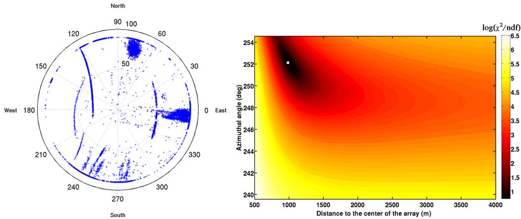
**Fig. 2. Left:** Arrival direction of the reconstructed events for one day of data taking. We can observe the trajectory of some planes and a large number of events near the horizon, that correspond to noise sources. **Right:**  $\chi^2$  evolution as function of the source position on the ground. This source is located at 252°(SW) and at 1050m from the center of the array (white dot).
